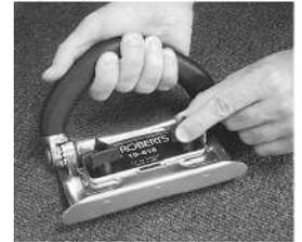
4. Tighten knobs firmly to secure blade holder.
