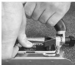
2. Squeeze the handle to open up the handle and disengage the teeth. Retighten the knob firmly after setting handle to the desired angle.
