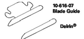
Follow instruction of contact cement's manufacturer for applying. After applying Delrin® to blade guide, apply pressure by clamping.
